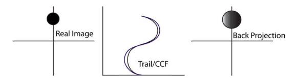
Figure 3.8: Left: An emission site in a real image  $(0, K_y)$ . Centre: The resulting trail from a point in the emission site (black), together with a sinusoid of similar velocity (blue). Right: A back projection of the trail without filtering. The image is blurred due to contamination with similar sinusoids.
